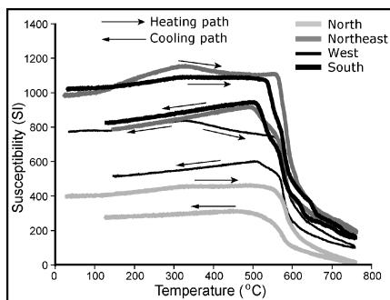
**Figure 4.** Susceptibility vs. temperature plots showing heating and cooling paths for selected Great Eucrite samples (one from each traverse).
