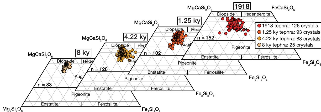
**Figure 3.** Compositional data from the analyzed Katla tephras are plotted in the “pyroxene quadrilateral.” Katla pyroxene compositions are confined to the diopside and augite fields for all four of the investigated tephra units.
