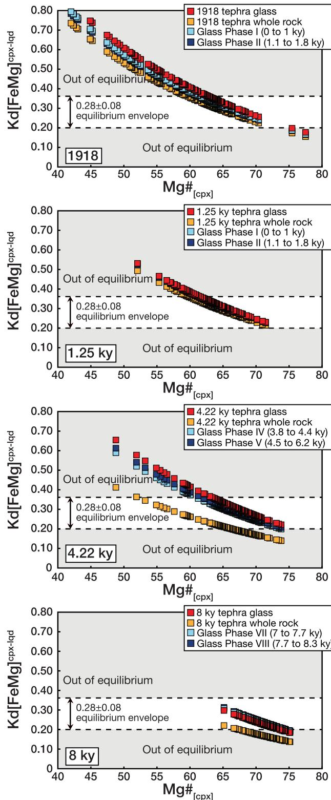
**Figure 5.** Pyroxene compositions and possible equilibrium melts in a test against  $Kd[FeMg] = 0.28 \pm 0.08$  [Duke, 1976; Putirka, 2008]. Data points that fall within this equilibrium envelope are taken to the next level of testing (e.g., Figure 6). The “out of equilibrium” data are discarded at this stage. Note, “Glass Phase” nominal melt data are from Óladóttir et al. [2008].
