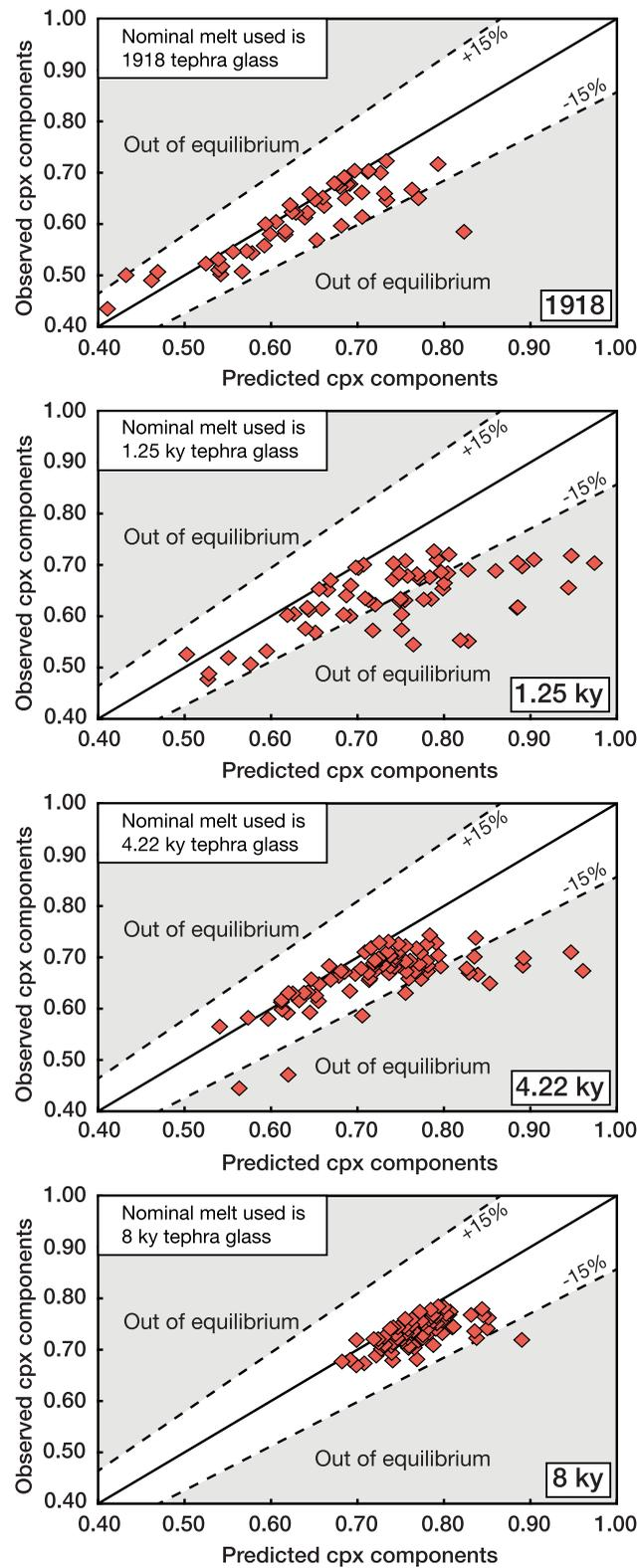
**Figure 6.** Observed versus predicted mineral components of diopside and hedenbergite for each Katla tephra sequence when paired with the best fit nominal melt. Values that fall within  $\pm 15\%$  of the 1:1 line (white areas) satisfy equilibrium conditions and are taken forward for final thermobarometric modeling [cf. Putirka, 1999, 2008].
