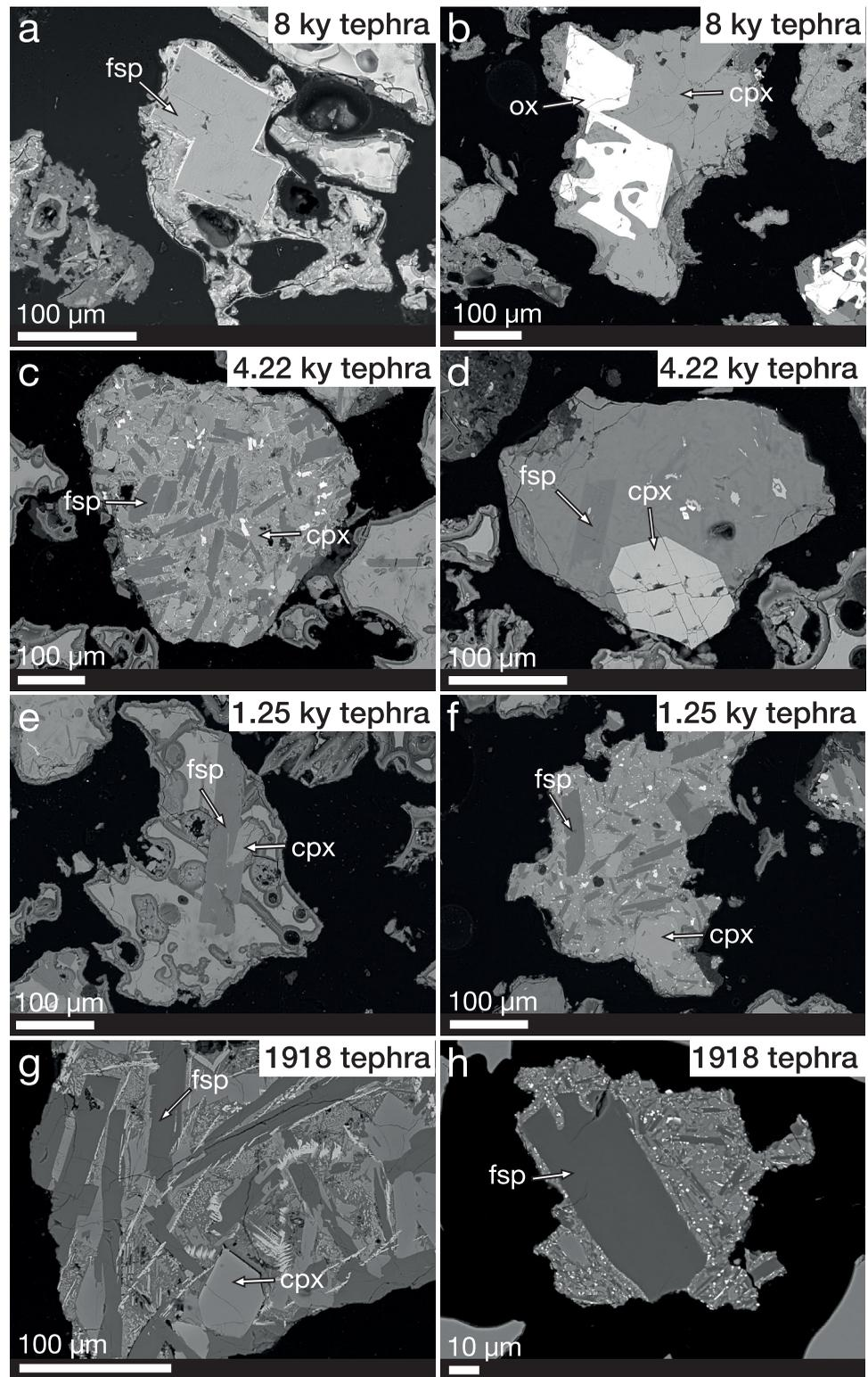
**Figure 2.** Representative back-scatter electron images of the investigated Katla tephra (8 kyr to 1918 AD). Minerals comprise mainly clino-pyroxene (cpx), plagioclase feldspar (fsp) and Fe-Ti oxides (ox), which occur in clusters and as free-floating crystals within the glassy groundmass.
