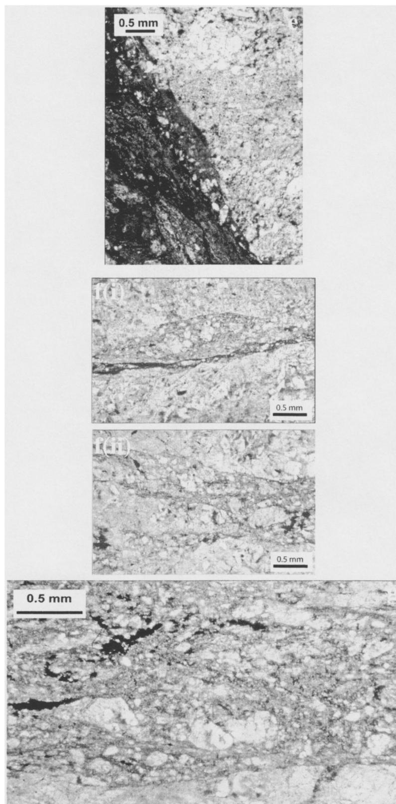
**Figs 4(e)–(g)**—(e) Thin section in PPL of crush zone rocks at ~218m, showing fine-grained cataclastic groundmass and igneous fragments; (f(i,ii)) Mylonitic tuffisite veins at contact (220m) in porphyritic microgranite (thin section in PPL); (g) Pervasive tuffisite veining with cataclastic crushing in damage zone near main contact (~218m; thin section in PPL). Note smeared our mafic enclave.
