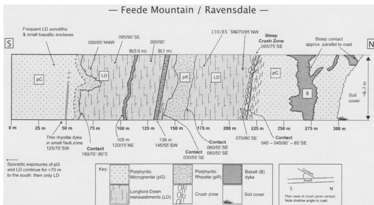
Fig. 2—Schematic log of the newly exposed road section at Feede Mountain.
