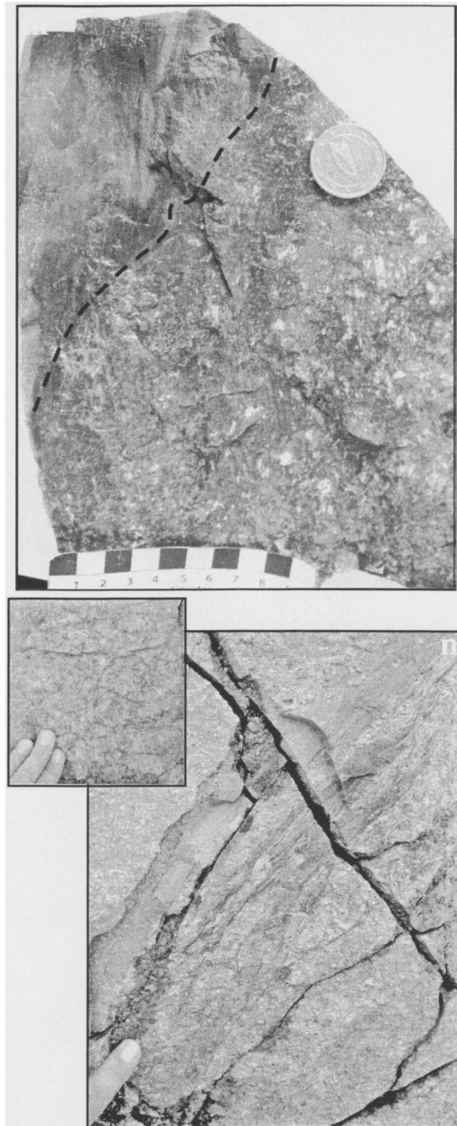
**Figs 3(m)–(n)—(m)** Crushed porphyritic microgranite at 218m contact. Note the very small grain-size and the absence of unbroken zoned phenocrysts and enclaves, implying severe physical crushing and intermingling. Samples taken from 2m north of the contact show regular grain-size again. Coin is 2.5 cm across; (n) Wide and extensive mylonitic tuffite veins in porphyritic microgranite near contact (~220m). *Inset:* locally pervasive tuffite veins near contact (220m).
